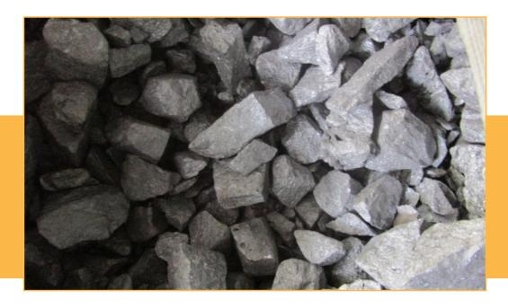
Ferro Silicon is a Ferro alloy composed of iron and silicon. It is used in steelmaking and foundries as a source of silicon in production of carbon and stainless steel.
